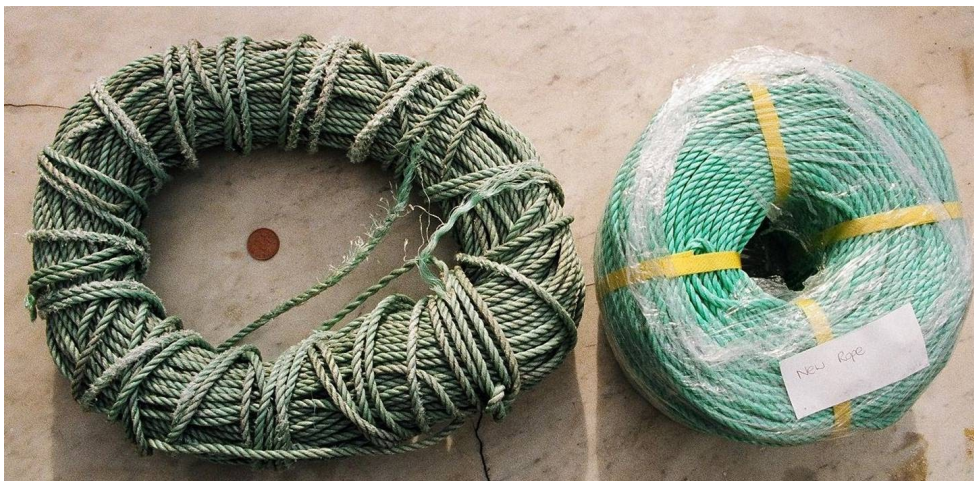
Effects of UV exposure on polypropylene rope. 20
