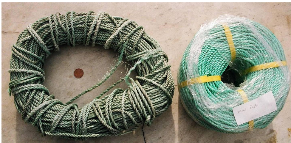
Effects of UV exposure on polypropylene rope. 20
